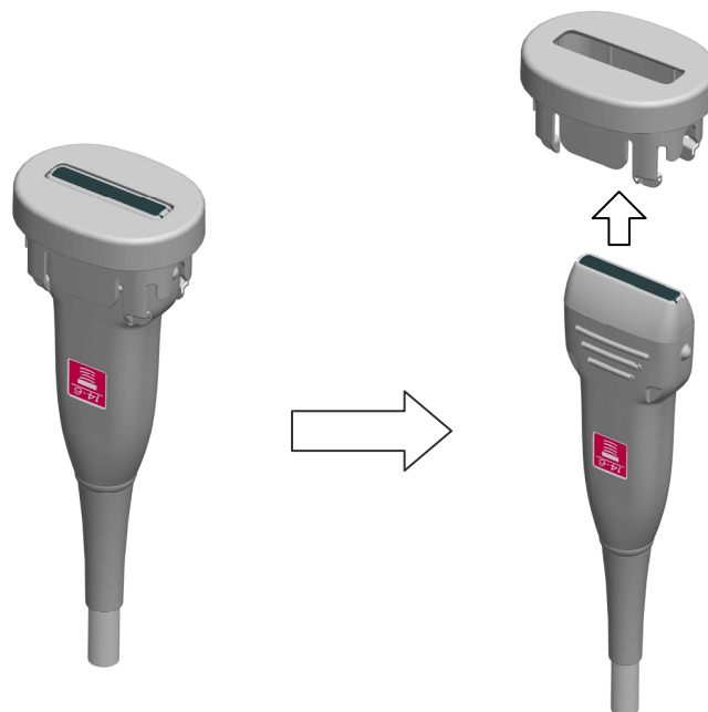
Fig. 14 How to release the Elasto coupler
