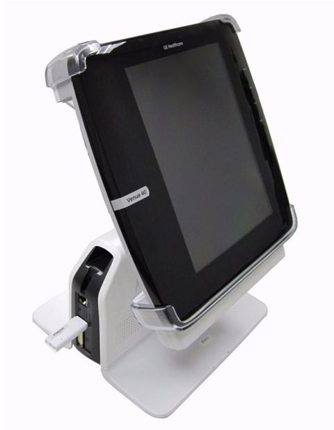
Figure 2-15. Wireless Network Card Connection
