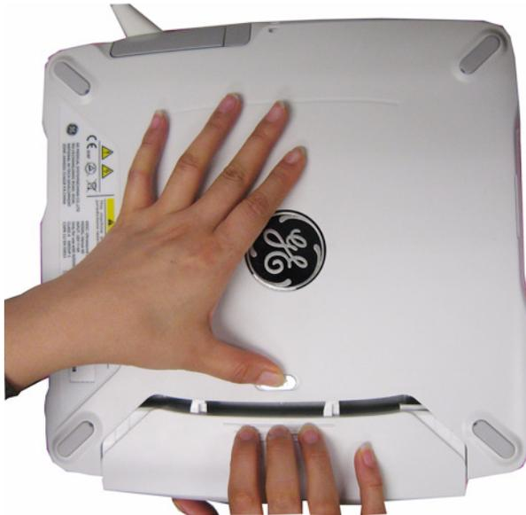
Figure 2-8. Battery replacement
