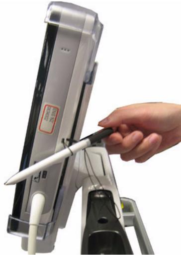
Figure 2-33. Thread through loop
