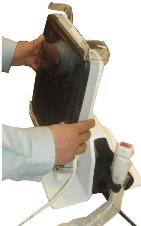
Figure 2-17. Mount to Docking Station/Docking Cart
