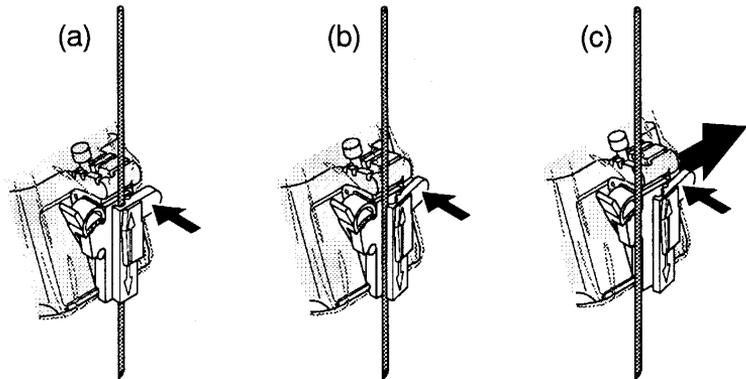
Figure 5-19. Release the needle from assembly
