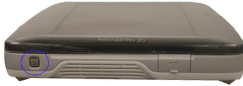
Figure 2-24. Power On/Off Switch Location
