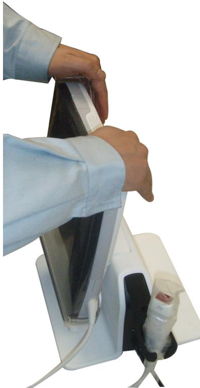
Figure 2-18. Mount to Docking Station/Docking Cart
