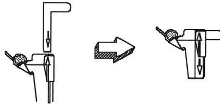
Figure 5-9. Needle Barrel Installation
