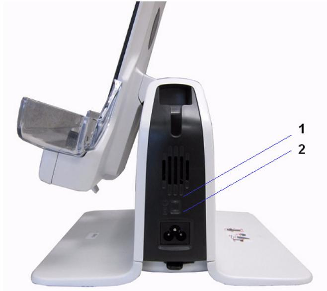
Figure 2-25. LED Indicators (Docking station/Cart)
