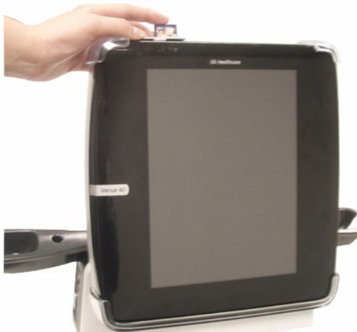
Figure 2-11. Insert SD Card
