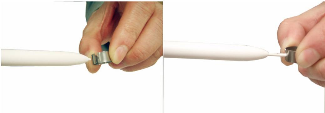
Figure 6-1. Stylus refill replacement
