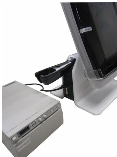
Figure 2-12. B/W Printer Connection
