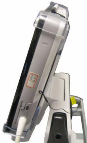
Figure 2-34. Stylus attached to Venue 40
