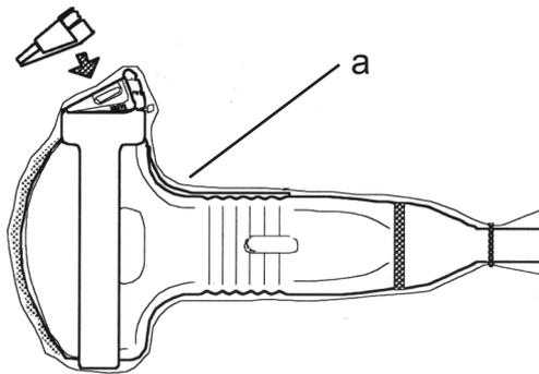
Figure 5-15. Fixing the Needle Clip Attachment
