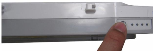
Figure 2-9. View battery capacity
