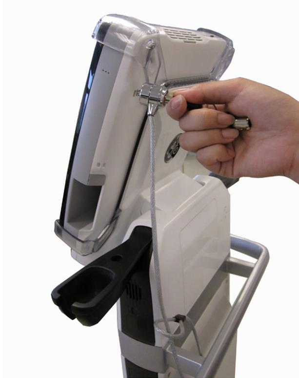
Figure 2-21. Insert the security lock
