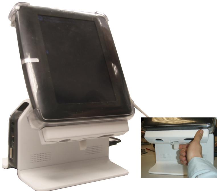
Figure 2-19. Release system from Docking Station/Docking Cart
