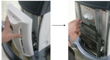
Figure 3-21. Air filter location
