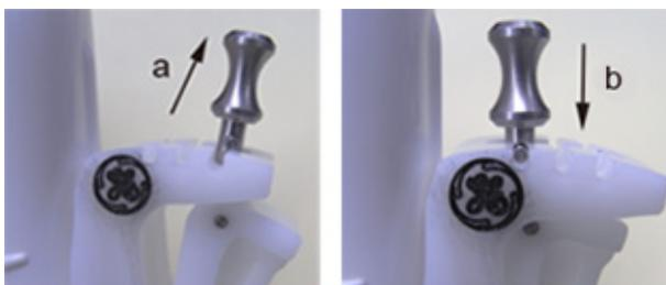
Figure 1-39. Pull up and push down the pin
