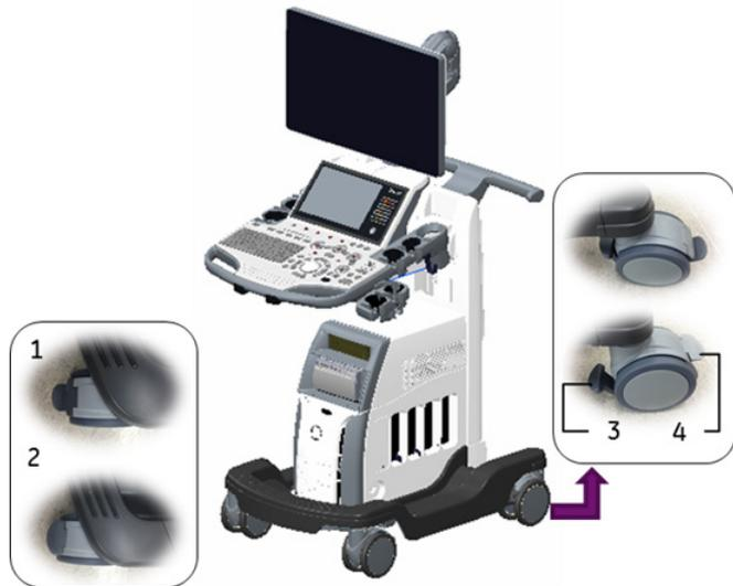
Figure 1-16. Wheel lock and Swivel lock
