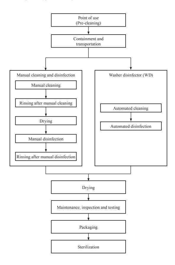
NOTE: Only the accessories are compatible with automated reprocessing according to the flowchart above.
