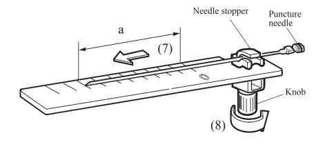
(9) Insert the puncturing needle until the needle stopper contacts the needle locking base. The tip of the puncturing needle reaches the target puncture region.
