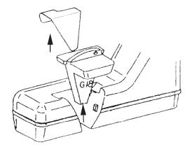
(3) To remove the lock plate, pull up its side as shown below.
