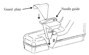
(3) Slide the lock plate to the front side. This locks the needle guide in place.
