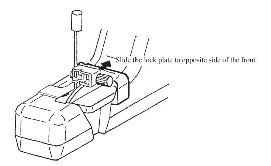
(2) Turn the needle 90 degrees. Lift up and remove the needle guide.
