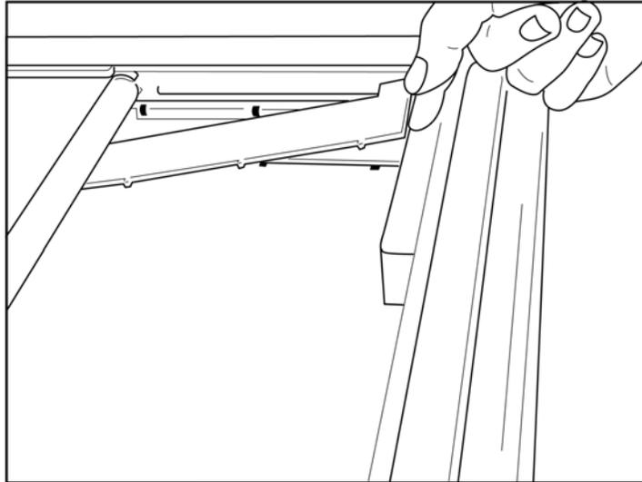
1. Slide paper tray spacer towards rear wall of paper tray. Align the bottom four plastic arms with the four openings in the base of the paper tray. Similarly, align the top 3 plastic arms with the three openings on the rear wall of the paper tray.
