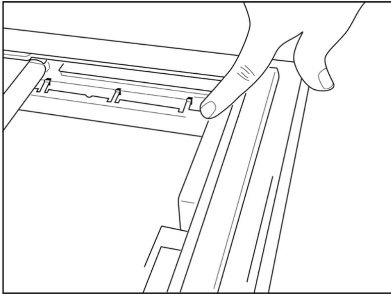
2. The paper tray spacer should be parallel with the rear wall of the paper tray.
