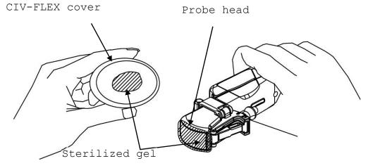
Fig. 13 Placing the gel
