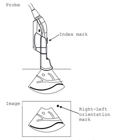
Fig. 4 Relationship between the directions of the probe and the Right-left orientation mark
