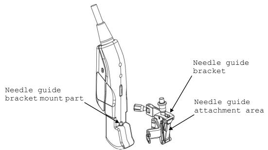
Fig. 11 Position for mounting the needle guide bracket
