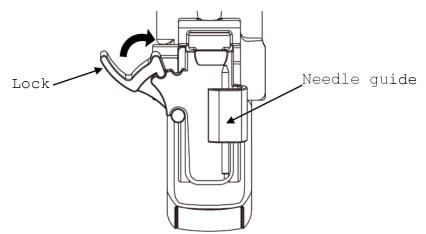
Fig. 15 Attaching the needle guide
