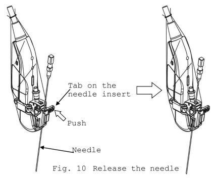
In the case of the CIVCO Ultra Pro  $3^{\text{TM}}$ , push the green quick release lever of the needle guide toward the bracket to open the needle insert, and then remove the needle.
