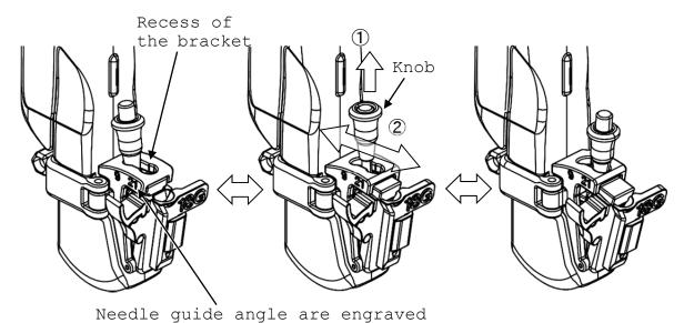
Fig. 17 Setting the needle guide angle
