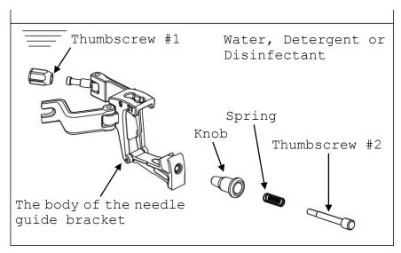
Fig. 22 Immersion of the Needle Guide Bracket
