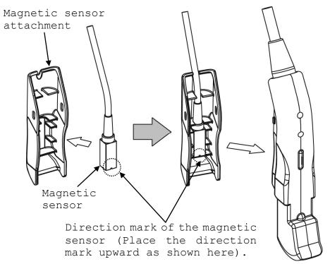
Fig. 7 How to attach the Magnetic Sensor Attachment
