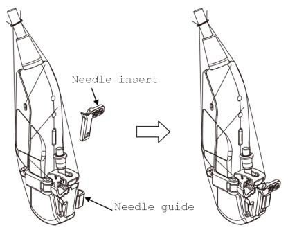
Fig. 16 Attaching the needle insert
