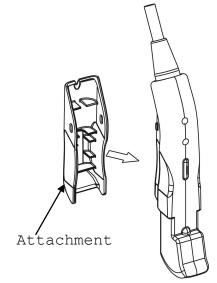
Fig. 5 How to attach the attachment
