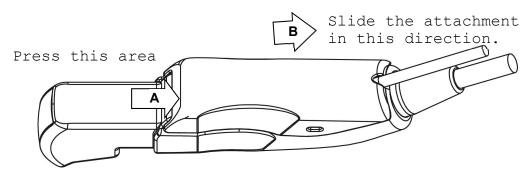
Fig. 8 How to release the attachment from the probe
