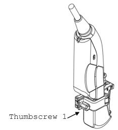
Fig. 12 Fitting the needle guide bracket
