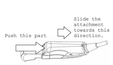
Fig. 6 How to release the attachment
