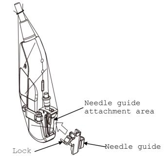
Fig. 14 Attaching the needle guide
